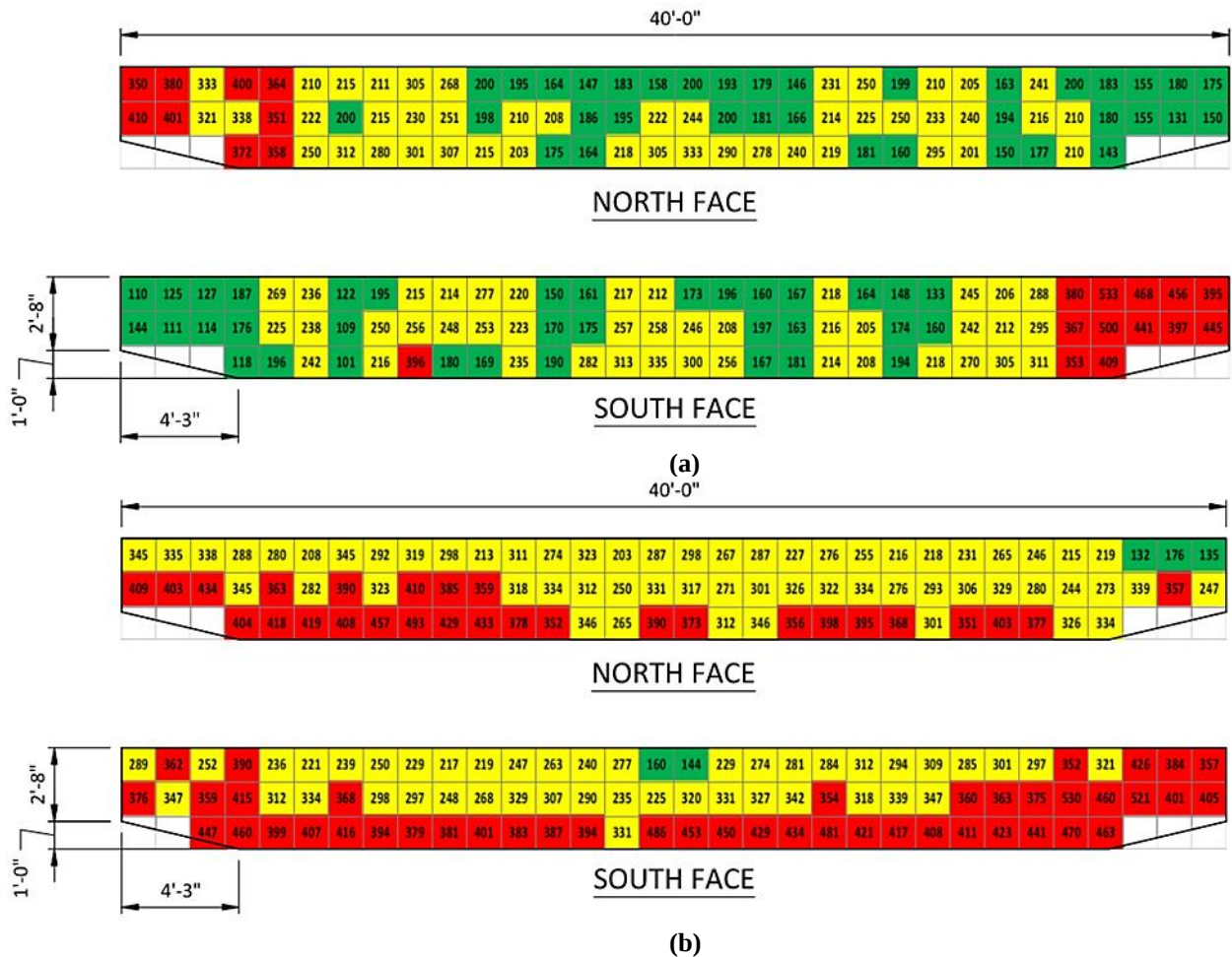
Figure 9. Half-Cell Measurements Using a 16-x-16-Inch Grid Pattern Show the Probability of Corrosion on the (a) Pier 1 and (b) Pier 3 Caps of the Route 629 Bridge. Numbers in each square are the magnitude of the half-cell measurement but are reported as positive values instead of the measured negative value (VDOT Contracted I-64 Bridge Substructure Studies Project, Route 629, 2021).
